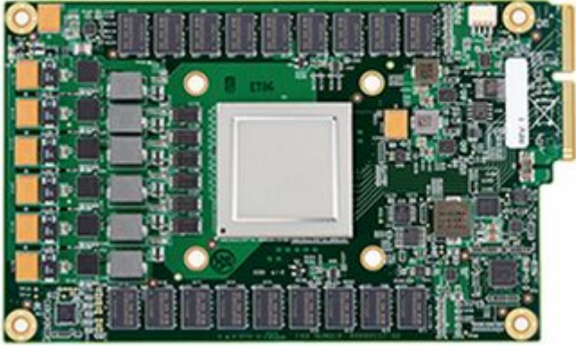
Google's first Tensor Processing Unit (TPU) on a printed circuit board (left); TPUs deployed in a Google datacenter (right)
